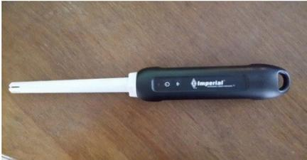
The thermal-hygrometer measures humidity, dry-bulb and wet-bulb temperature. With two humidity sticks and accurate airflow measurements, we can calculate the capacity of an air conditioning system.
