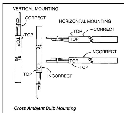
A lot of TXV's are misdiagnosed and replaced because of refrigerant flow control issues and all that really is wrong with the TXV is the "installation". Keep these little steps in mind when diagnosing TXV's problems.
