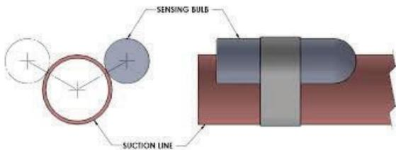
5% of bulb surface is in contact with the suction line the other 95% of bulb surface is exposed to supply plenum temperature.
