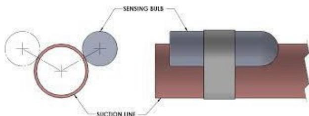
5% of bulb surface is in contact with the suction line the other 95% of bulb surface is exposed to supply plenum temperature.
