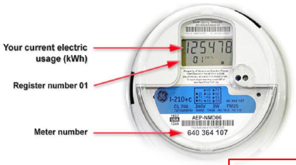
Figure 1: Typical utility meters and identification number
