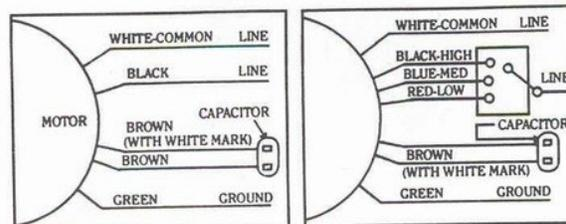
Permanent-Split Capacitor motors have many different kinds of wiring arrangements. The standards for FASCO and most other manufacturers is shown.
